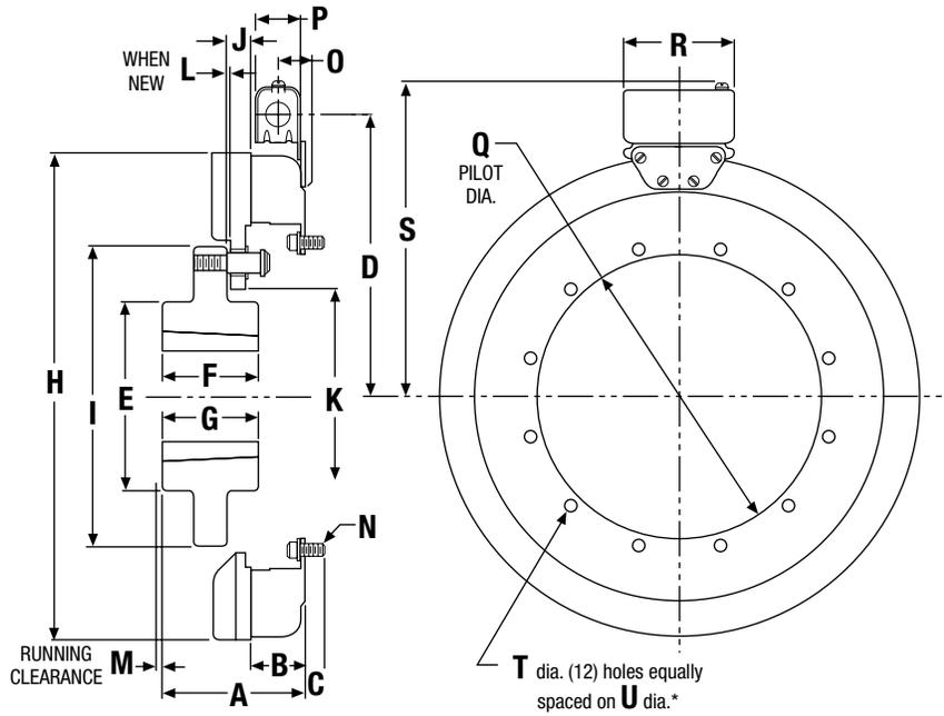
\*Mounting holes are within .010" (.254) of true position relative to pilot diameter.
